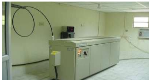
Figure 1. Solid state Nd: YAG Laser source at WRI used for experimental work [18].
